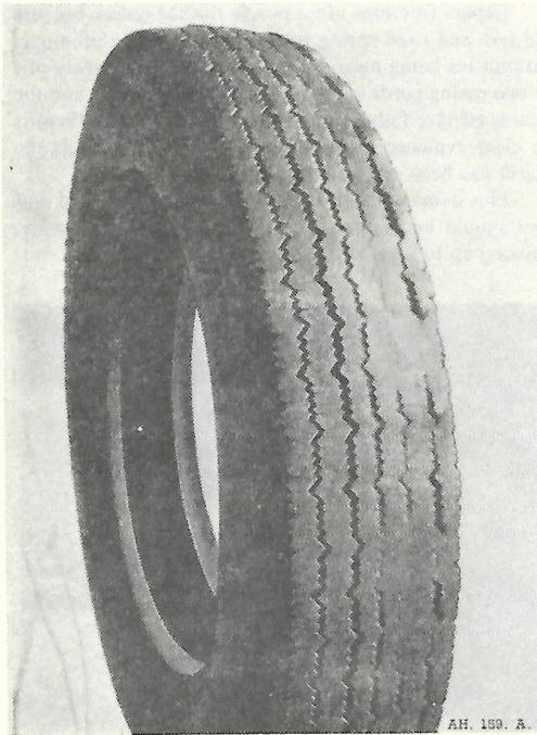
Fig. O.17. Irregular "Spotty" wear, to which a variety of causes may contribute.
