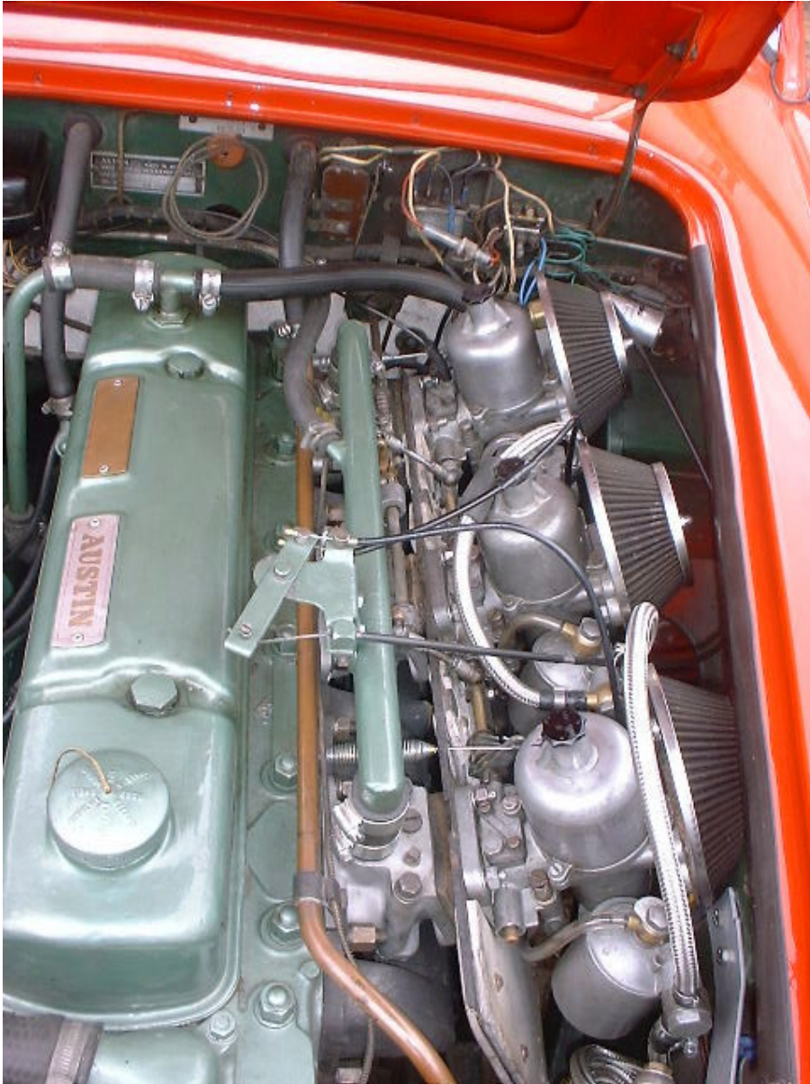
HD6s view two. Only two chokes are actually connected!
