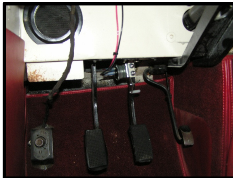
Assembly installed on Ventilator Door Surround. You should be sure to open the door as you install this or it may prevent the door from opening.
