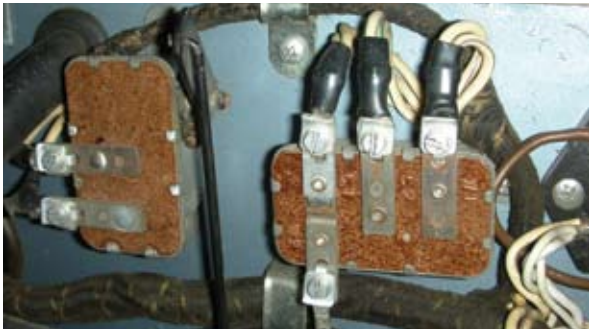
The throttle switch (left) with the lever connected to the throttle linkage, and the overdrive relay (right) on the firewall of the 6-cylinder Healeys. On the BN2 the relay is located at a position just below that shown..
