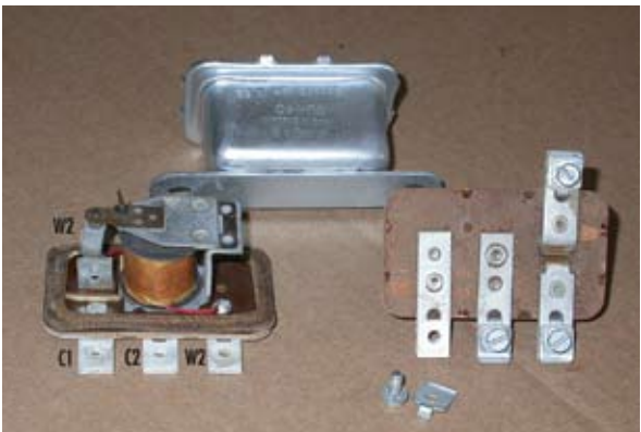
The overdrive relay, with the case open so we can see how the coil is wired and how it closes the points to connect the C1 and C2 posts. The exterior of the base plate from a second relay is shown at the right.
