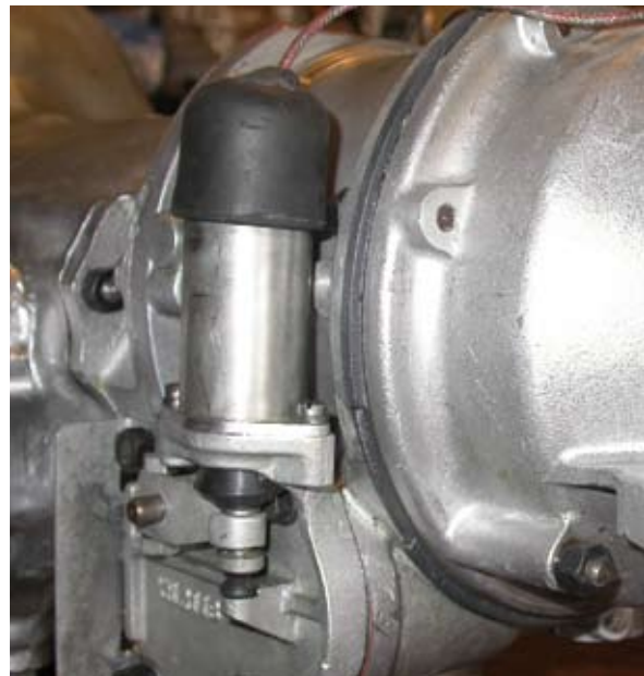
The overdrive solenoid with the exposed operating lever configuration. This first appeared during BN1 production and continued through the 100-Six models.
