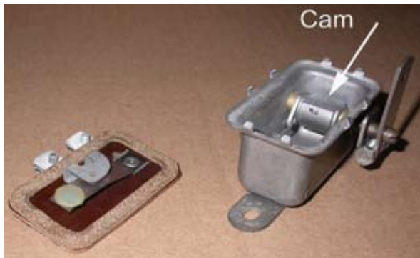
The throttle switch with the case opened. In this view, one can see how adjusting the throttle lever will determine when the throttle switch is engaged.
