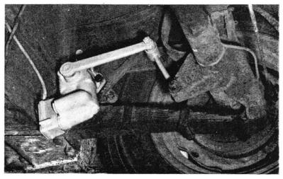
capacity over the conventional shock absorber. (Modern suspension systems often overload the capacity of the shock absorber by their very low spring rates.) The Firmaride units are flexibly designed for use with adjustable units so that the car can be set up to the best advantage.
