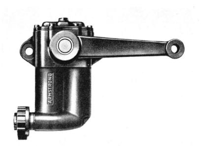
described as a damper. The springs should absorb the initial shock from the bump, and the damper controls the bouncing effect. With leaf springs the friction between the leaves acts in a damping capacity and partially removes the need for a separate damper or shock absorber, as it is known more often in the United Kingdom.
