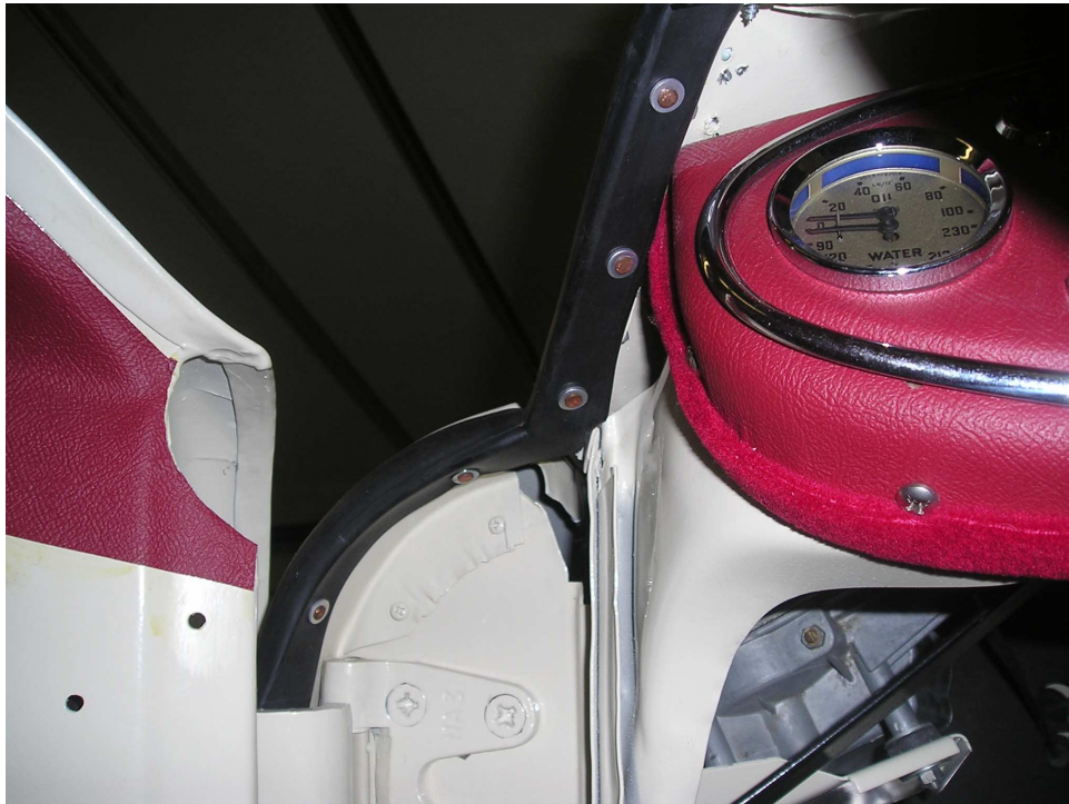
This Photo gives under side view showing split rivet heads with flat washers. Also shows relation of seal which ends behind upper door hinge.
