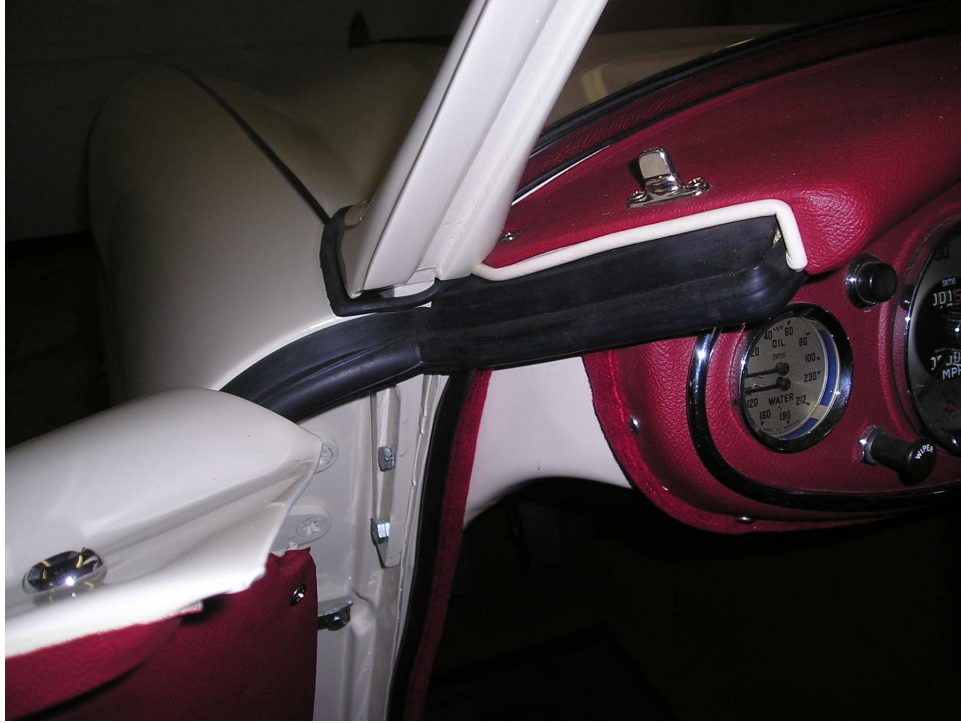
This Photo shows windscreen now in place but final black sealant has not yet been applied.
