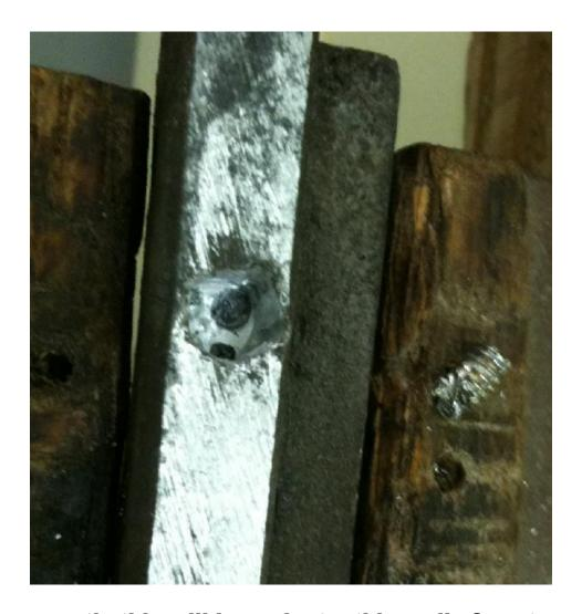
Done correctly this will leave just a thin wall of post on either side of the hole. Next slide the Rivnut, flange first, into the hole.
