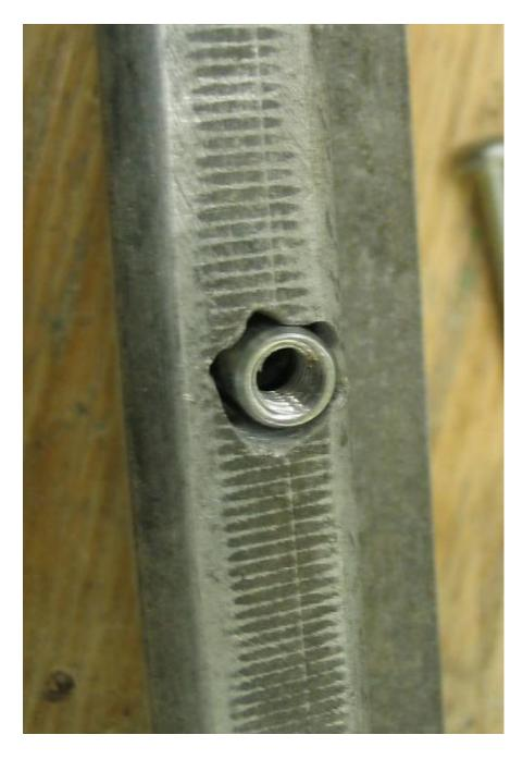
When The Hole is Deep Enough The Top of The Rivnut Will be Flush With The Post Surface
