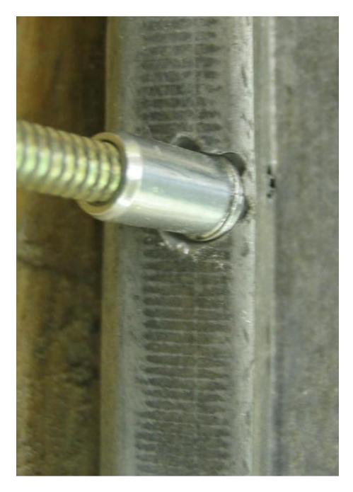
The Flange Has to be Small Enough To Fit Into The 5/16" Hole
