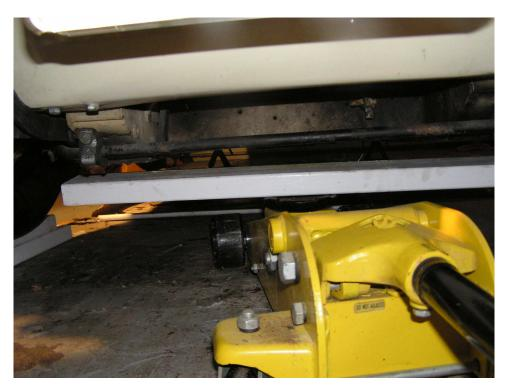
5. When the car is as high as needed, place the front Jack Stands under the 2 x 4 and lower the car and 2 x 4 onto the Jack Stands. The Stands should be as far apart as possible but not so close to the suspension that movement is restricted. I use stands with saddles wide enough to nest a 2 x 4 into the saddle.
