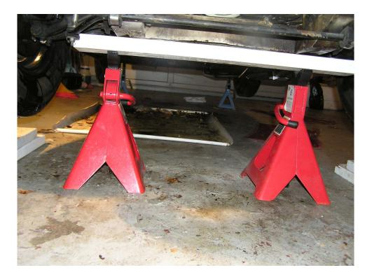
6. Using this method, I can move the front wheels with either the steering wheel or just by turning the brake drum side to side by hand to get at various items that are being worked on. And, the Jack Stands do not get in the way of any other work being done under the car.
