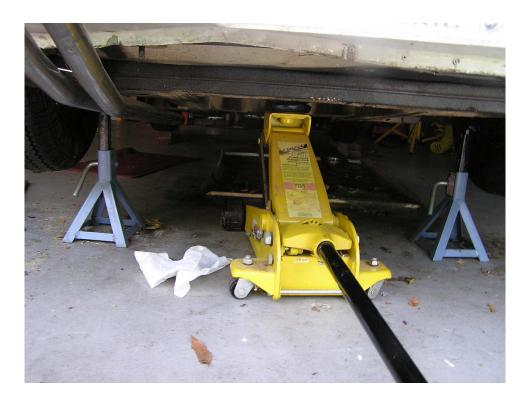
4. Go back to the front and use a 2 x 4 cut long enough to span from frame rail to frame rail at the front Crossmember. Place this on the Garage Jack Saddle between it and the Crossmember and jack the car up to the proper height. Photo Four.
