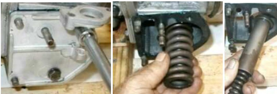
The speedometer bearing & pinion were removed next. This need be removed only if one plans to disassemble the rear casting to replace the two rear bearings. The retaining bolt was removed first, and then the nut from the end of an old speedometer cable was screwed onto the speedometer bearing and a large screwdriver was then used to pry against the lip of the speedometer nut to remove the bearing (left photo below). The parts in right photo were bagged together.
