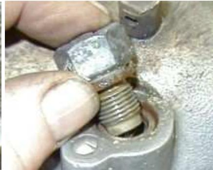
The operating valve components are shown below. The plug and copper washer are new replacements.
