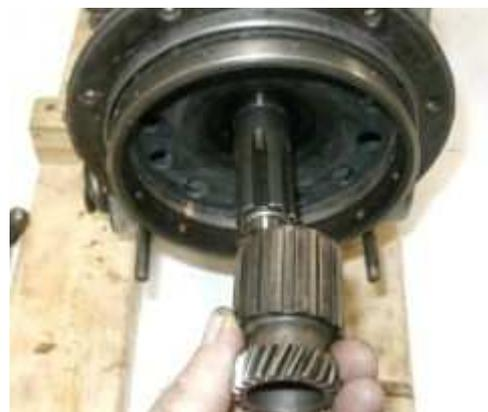
**Removing Main Casting:** The nuts and lock washers from the two bottom studs were removed first. Next, the nuts on the two top studs were loosened; these nuts can't be removed until the main casting is
