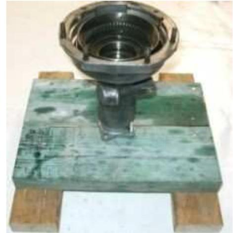
**Annulus End Float:** The annulus end float was measured before the rear casting was disassembled. The end float is adjusted by changing the adjusting washer between the rear bearing and a shoulder on the annulus shaft. If the end float is within spec before disassembly, then it should be within spec even if new bearings are installed because the bearings are made to a very close tolerance.
