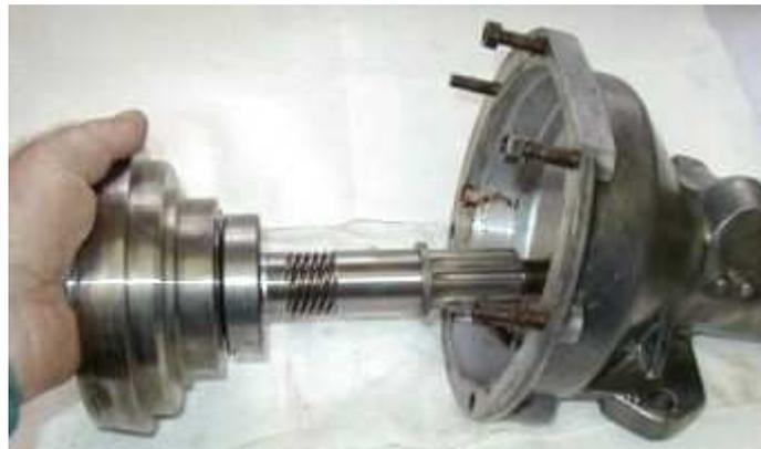
**Middle Bearing removal:** This bearing is also known as the annulus head bearing. A large bearing separator (available from Harbor Freight, ~\$20) was used to first push the bearing away from the shoulder on the annulus by tightening the two black bolts in the left photo below. Next, the bearing was pulled along the shaft by tightening the nuts on the threaded rods. The right photo shows the bearing nearly off the shaft. The press fit is only on the shiny section very near the shoulder.
