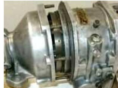
After the rear casting was removed, the planet carrier with planet gears and then the sun gear were removed as shown below. The planet carrier was cleaned and the bearings in each planet gear were tested by rotating the gears. All three gears rotated smoothly and there seemed to be no play in the bearings. It was decided that the planet bearings would not be replaced so it was not necessary to disassemble the planet carrier further.
