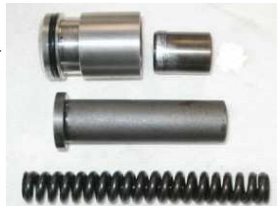
It is possible to replace the earlier accumulator with the later accumulator (the housing, piston, spacing tube and spring are all required). The Victoria British Catalog suggests this option if replacement springs, piston or rings are required for the early accumulator.
