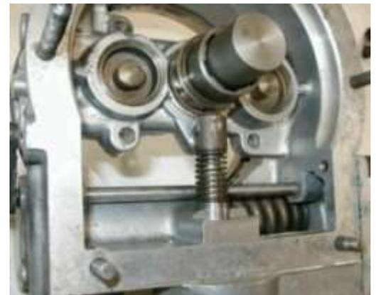
The second photo shows the pump components. The pump body is top left with spring and then piston below it. The pump body is pressed into the main casting and secured with the two screws. The spring is used to force the piston up --- the mainshaft cam forces it down. The lower end of the cylinder is sealed with the large threaded pump body plug in the upper middle. The screened cup is a filter secured to the plug by the screw in the lower right.
