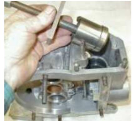
Oil from the pump goes through a passage in the main casting into the bottom of the accumulator cylinder. As oil is pumped in, the piston is pushed out of the cylinder compressing the two springs. The pressure builds as the springs are compressed.
