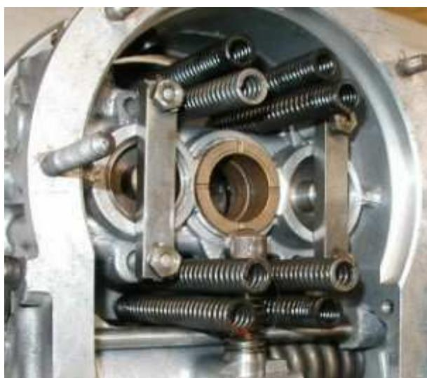
The two bars are held to the thrust ring pins by nuts are called bridge pieces. When the OD is switched to the engaged position, fluid enters the rear of the operating piston cylinders and pushes the operating pistons forward into the bridge pieces and then pushes the bridge pieces and connected thrust ring and clutch forward until the front cone clutch mates with the brake ring.
