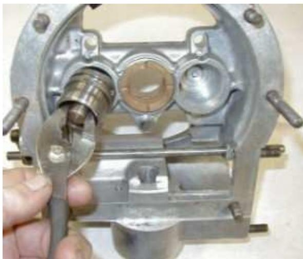
The piston shown is the earlier design with steel rings. The later design uses a rubber O ring. Both type of pistons are shown in the middle photo. Replacement steel rings are no longer available but the new design piston with O ring can be used in the earlier #22/1374 model but not the #22/1275 because it used smaller operating pistons.
