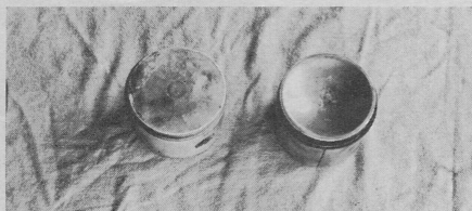
By using flat-crown Merryman piston, at right, a compression of 9.3:1 was obtained. Piston uses stock American rings.
