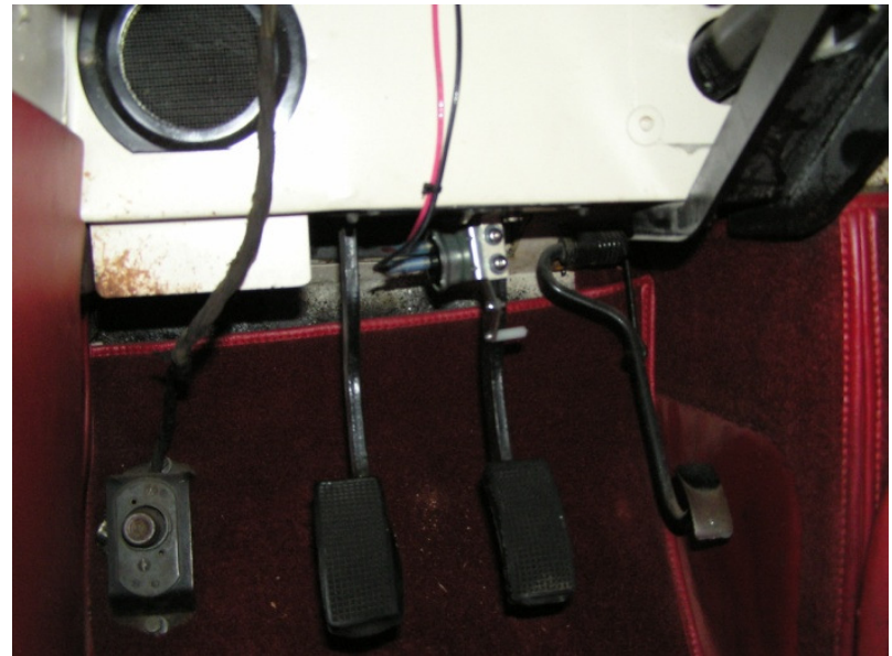
Assembly installed on Ventilator Door Surround. You should be sure to open the door as you install this or it may prevent the door from opening.
