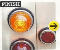
Reconnect the battery (preferably via an inline fuse) and check your hazard flashers work. Then, make sure the indicators are still working as before. If all these checks are okay, the install's complete and you're good to go. Reconnect the battery properly.
