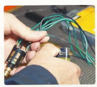
The warning lamp in the switch needs an earth. This can be connected by splicing to an existing earth wire. Alternatively, you can fit a ring terminal to the cable and connect via an existing earth point, or via a self-tapper into the car's metal structure.
