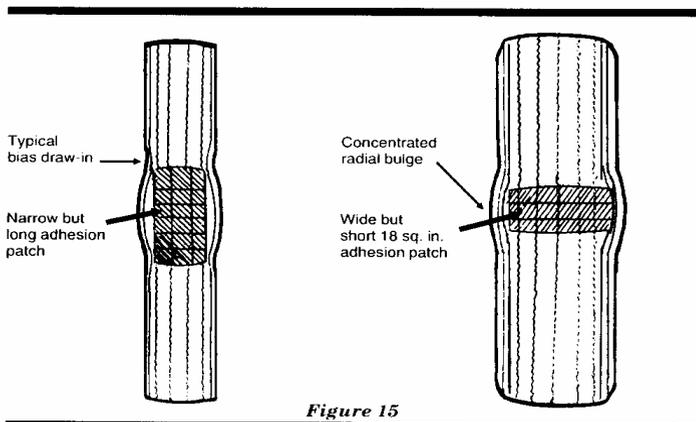
The above illustrates the tire patches of 18 square inches each: One on a four-inch wide tread and the other on an eight-inch wide tread.
