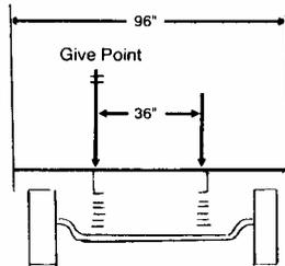
Common front leaf-spring motorhome suspension; it has a poor 1:2.6 ratio
