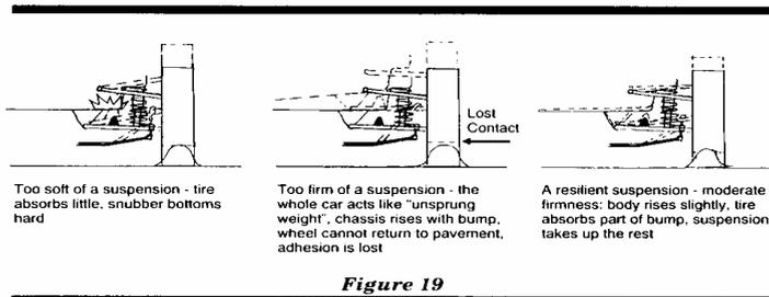
little understood subject of sprung versus unsprung weight. The idea here is that the more weight you have leaping up and down with the wheels, the harder it will be to keep it moving exactly with the road surface; thereby, maintaining adhesion; and obviously, the more it will bump the body up and down via the springs and shocks.
