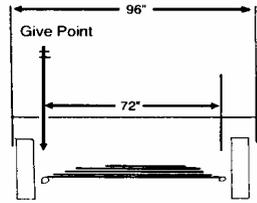
FMC, by using a Single Transverse front spring gave it a 1:1.3 ratio
