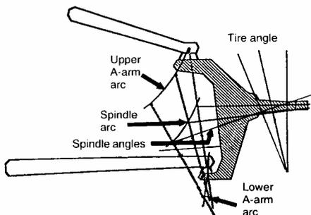
**Illustration of wheel tilt induced by geometry of suspension accelerating at extreme deflection. This is added to body roll deflection.**
