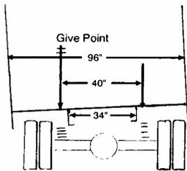
This typical truck/motorhome Suspension has only a stability to support ratio of 1:2.18
