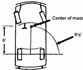
In a 180° turn that takes 4 seconds to complete, the center of mass must be accelerated through a 9½' arc in 2 seconds.
