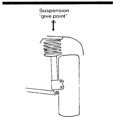
"Strut" suspensions can have very good "suspension width" giving approximate stability to support ratio of 1: 1.4
