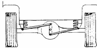
Note that this watts link allows vertical movement of either wheel but locks out any lateral movement of the body and it generates no side thrust.
