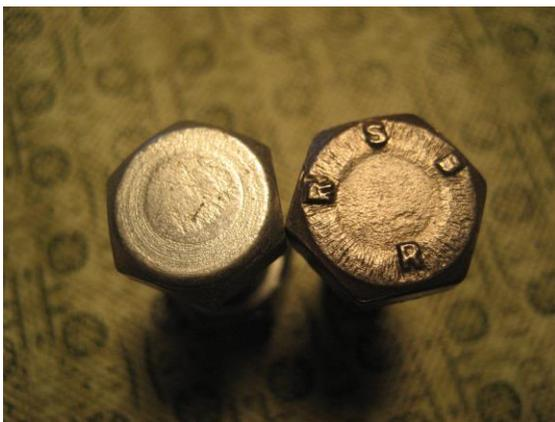
*RSB-Regis Screw and Bolt w/ "R" strength rating. UNC bolt on left has no marking so it's a Grade 2*
