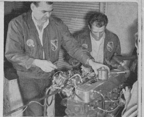
Verne Houle, left, Chick Vandagriff, right, take a high rpm reading. Tach, visible behind Houle, reads 7000 rpm.
